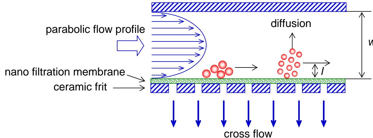
*separation is based on the hydrodynamic diameter of the analyte particles*
