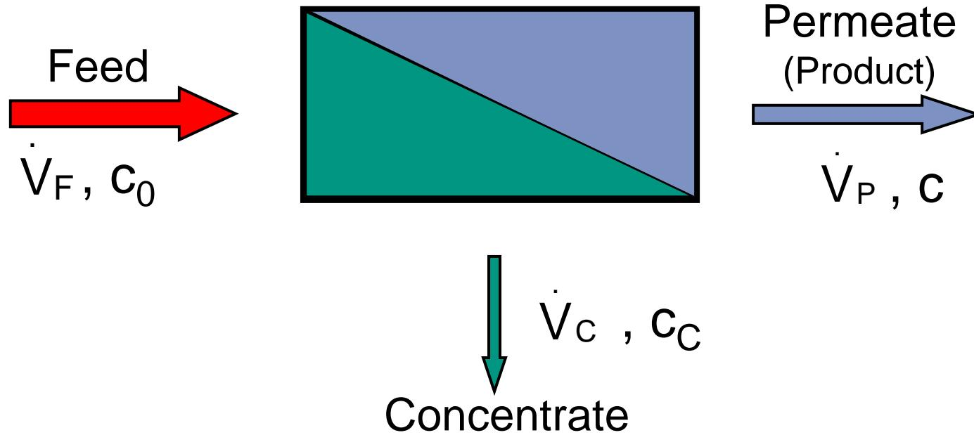
$$\text{Rejection coefficient } R = (c_0 - c)/c_0$$
